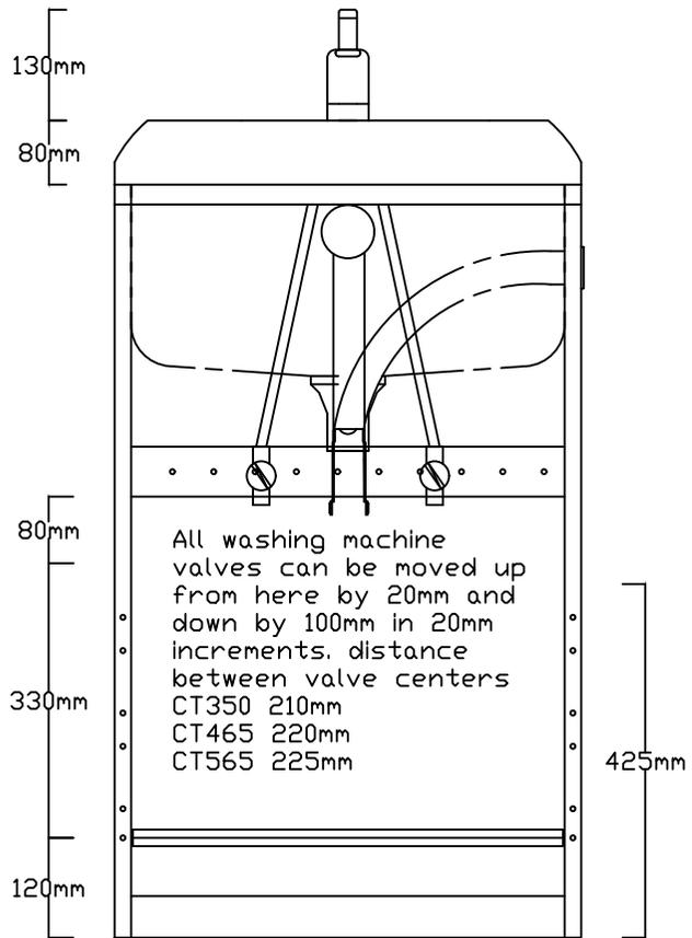
Basin size shown is for 565 wide STP 465 and 350 wide basins reduce accordingly to scale. use front view dimensions for widths.
